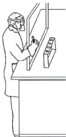
Figure 1 Example of suitable PPE for working with glass tubes under pressure.
